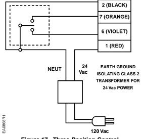
Figure 17. Three-Position Control.
